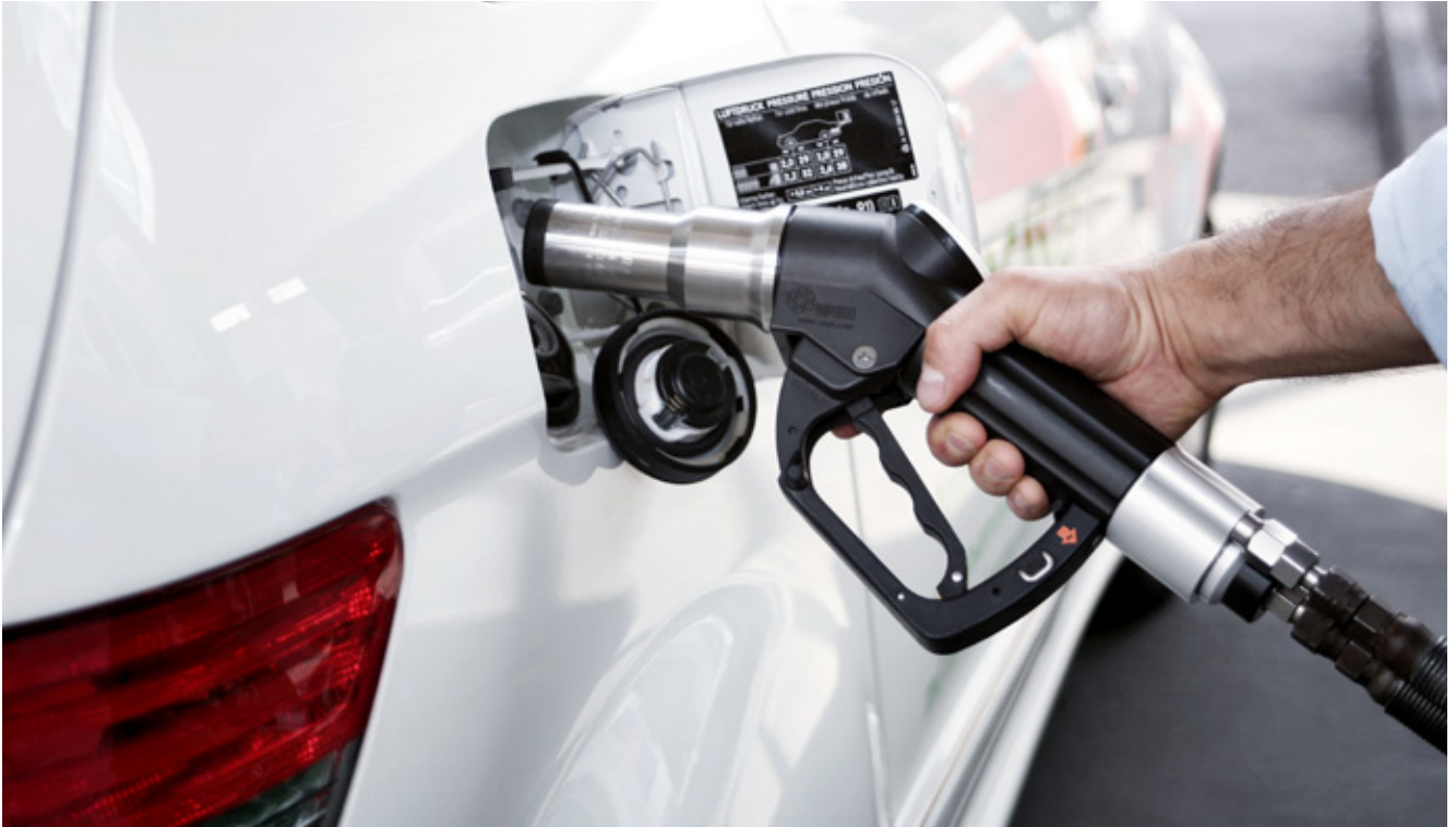
Car refuelling with TK17 CNG
